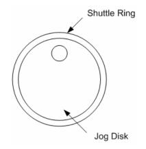
While playing back recorded video, users can rotate the shuttle ring to select different speed of forward and backward playback. Rotating the shuttle ring clockwise/ counterclockwise causes the unit to playback faster forward/ backward. According to the rotating angle the shuttle ring, users can choose the playing speed from 1×, 2×, 4×, 8×, 16×, and 32×, in both forward and reverse directions, shown as below figure:
